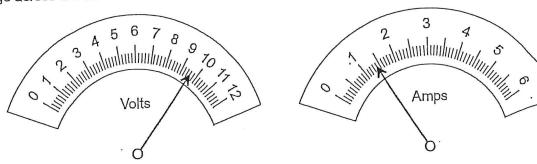
Determine the resistance R of the fuse wire,
