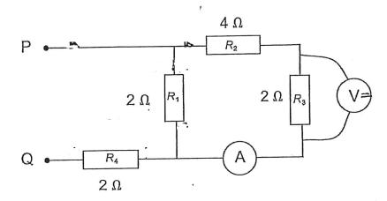
(a) Show that the total resistance between terminals P and Q is  $3.50\Omega$ .
